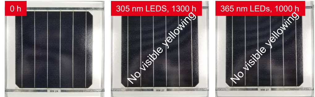
Visual inspection UV ageing under UV LEDs
