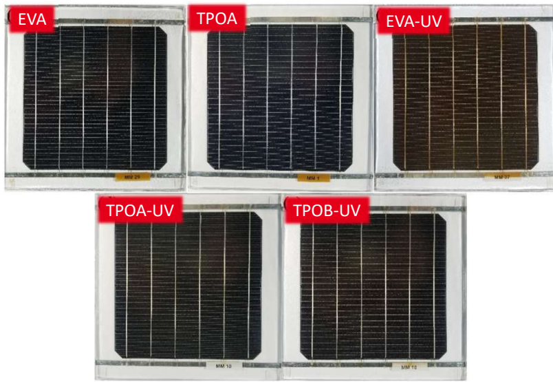
Front side of the mini-modules after 4200 h
