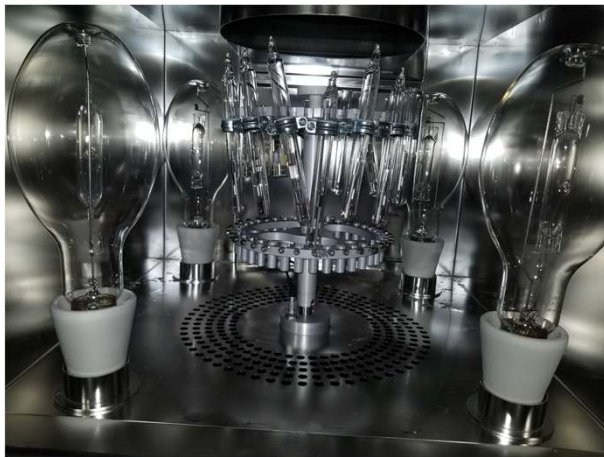
Samples sealed in glass capsules in UV chamber
